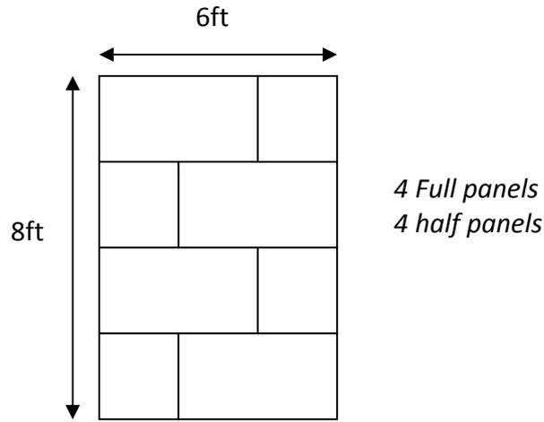
By designing the floor the long-side first, you use less half panels yet the floor is the same size 24ft<sup>2</sup>.
