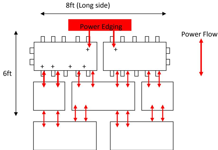
Regardless of most sizes, this power flow principle applies. This system therefore ensures that power flows to all the floor panels even if one panel is not receiving the power as it should for some reason (See trouble shooting guide if you are experiencing trouble with your floor)
